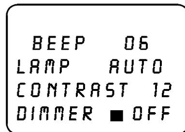
**PUSH** **(ENT)** to accept the data and return to a standard display. Alternatively **PUSH** **(CLEAR)** to abort entry or **PUSH** to move to the next item on the config menu. Refer to pages 106 - 107 of the operating manual.
